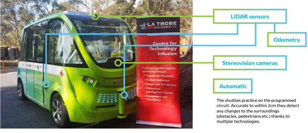
The NAVYA ARMA-4 Autonobus used at La Trobe University during this pilot project.
